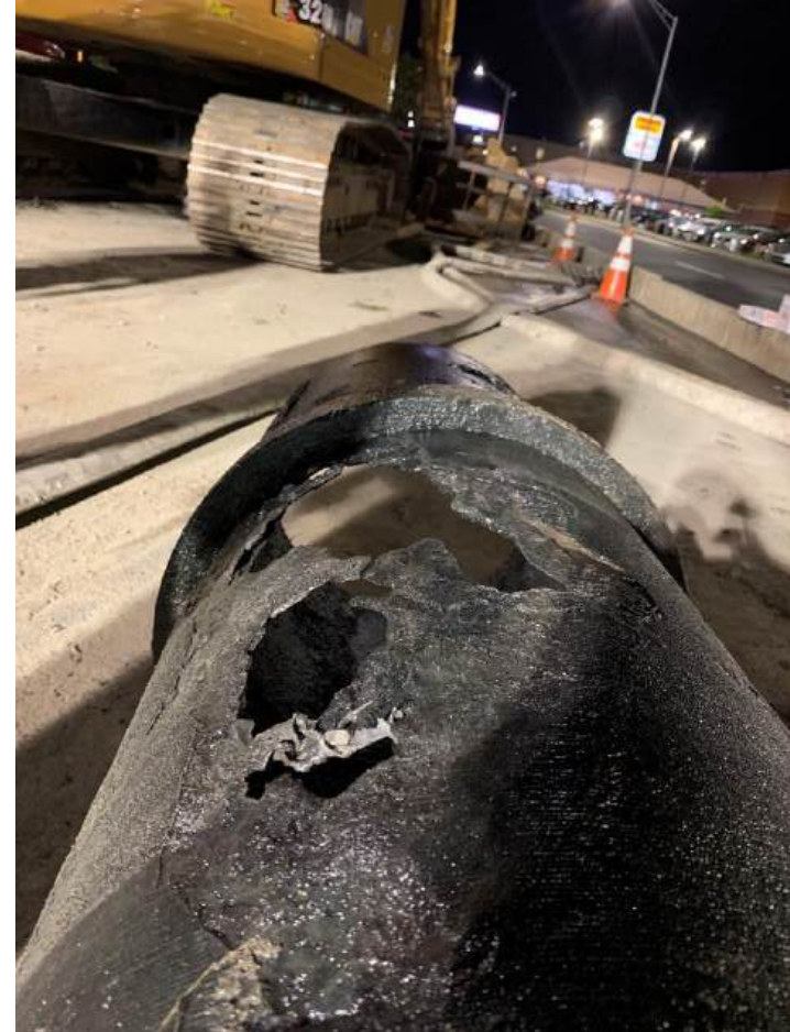
Break caused by Electric (Stray Current)
