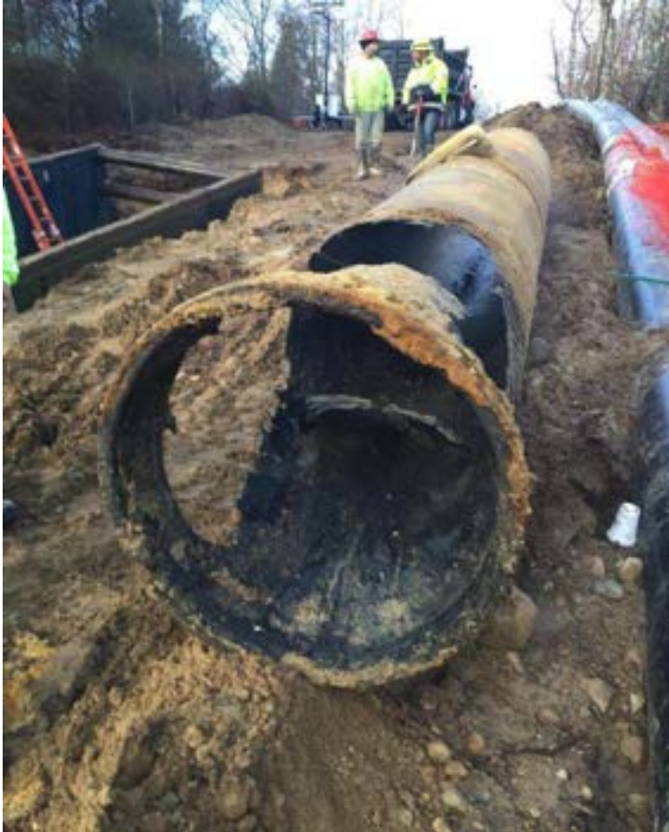
Break due to Hydrogen Sulfide
